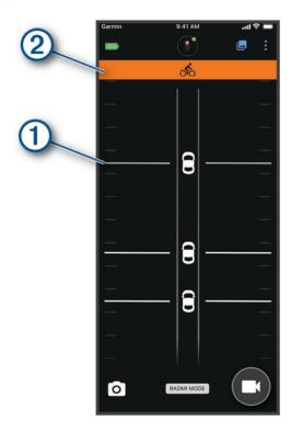
The vehicle position ① moves up the screen as a vehicle gets closer to your bike. The threat level banner ② changes color based on the potential level of threat. Green indicates no vehicle is detected. Amber indicates a vehicle is approaching. Red indicates a vehicle is advancing at a high rate of speed.
